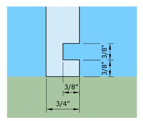
For added strength and ease of alignment, I used a dado to join the bottom to the sides.
