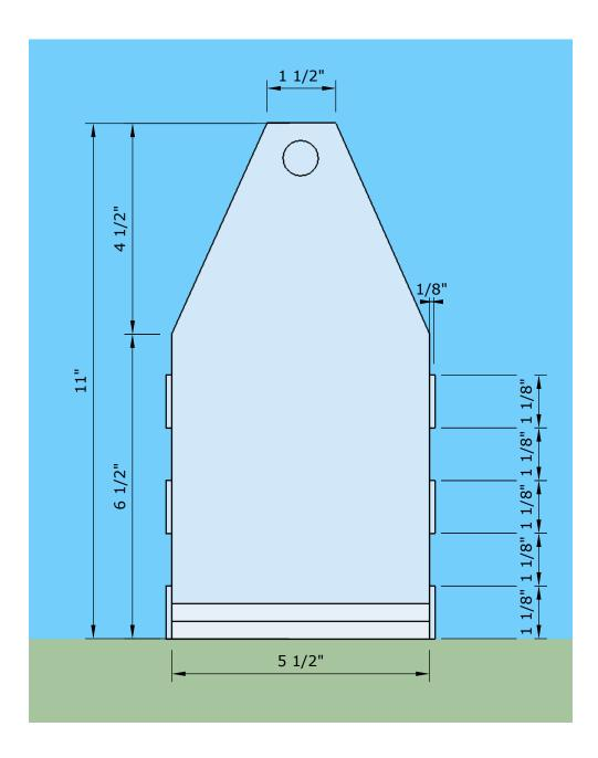
I cut six 1/8" slats from 5/4 pine (1 1/8" thick). Cutting thin wood is challenging, even with a table saw.
